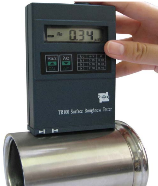
Figure3.8 TR100 Surface tester for measurement of surface roughness
