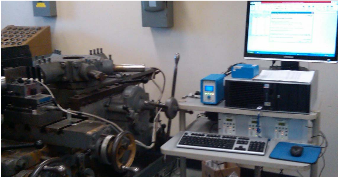
Figure 3.6 Complete set up of force acquisition system
